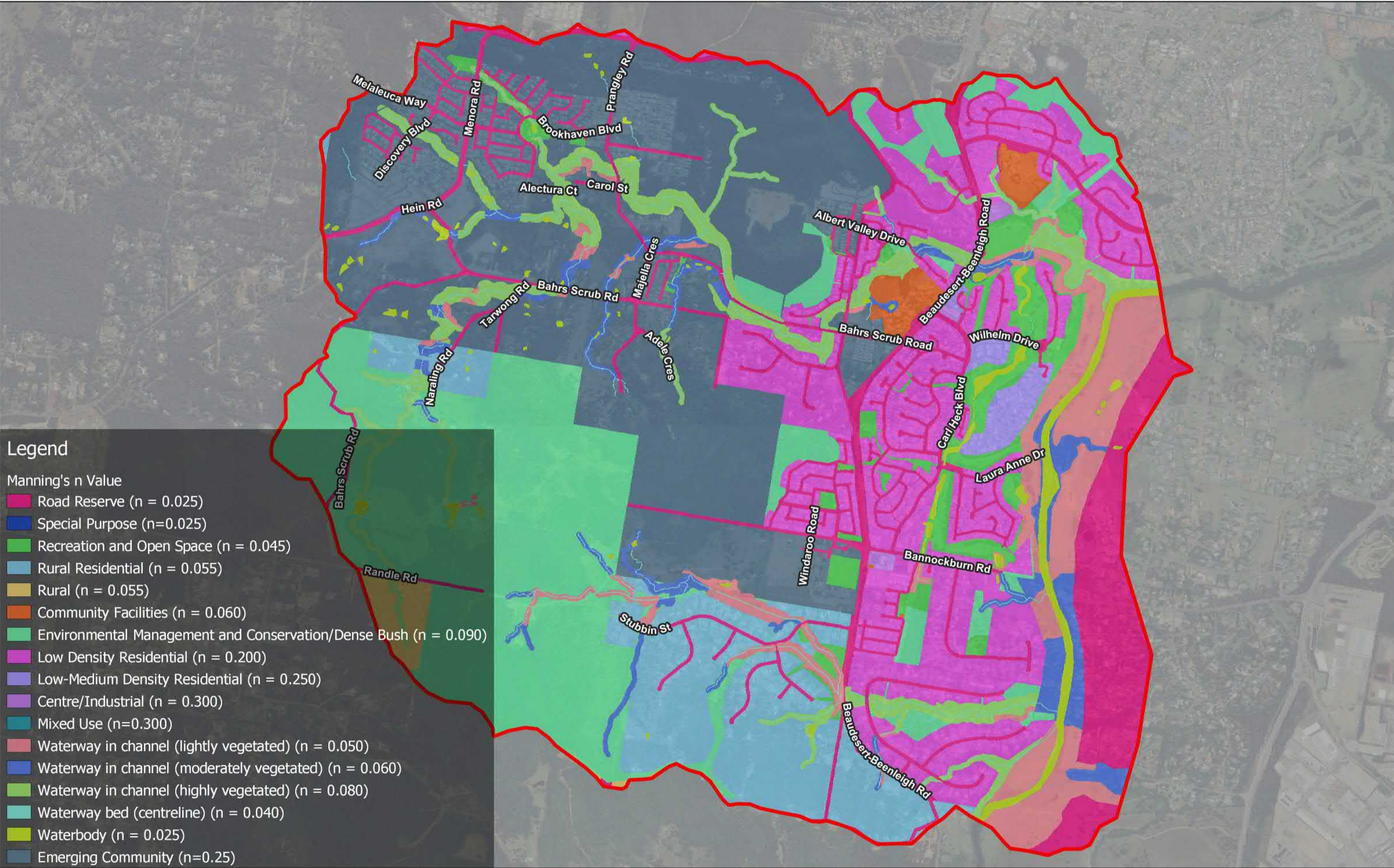
Figure 6.6 Windaroo Creek Flood Study TUFLOW Hydraulic Roughness - Design Events Drg Ref. M9000_082
